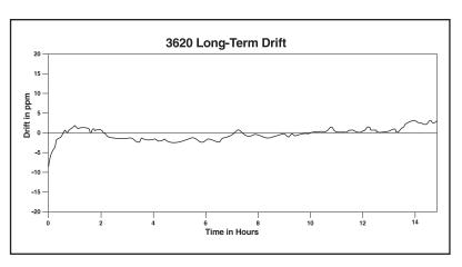
The 3620 performs with -10ppm drift (after 30 minutes) and 0.2% constant power stability.
